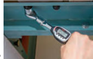
Combination example with ratchet head
