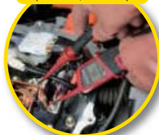
Voltage measurement prior to work is specified in the manufacturer manual.
